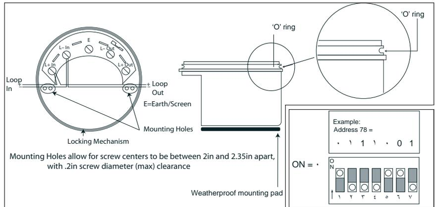
Fig 1. Wiring diagram
