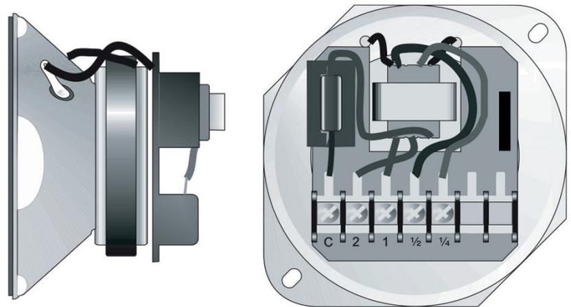
Desired wattage is selected by wiring into the corresponding terminal on the speaker terminal block.
