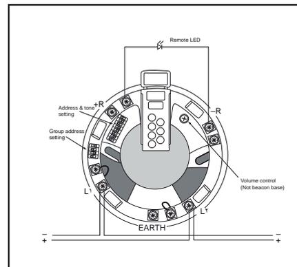
Fig 3. Base Wiring Diagram
